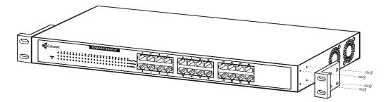
**3** With the assistance of another person, hold the switch in place in the rack and secure with two screws and nuts on each side (provided.
